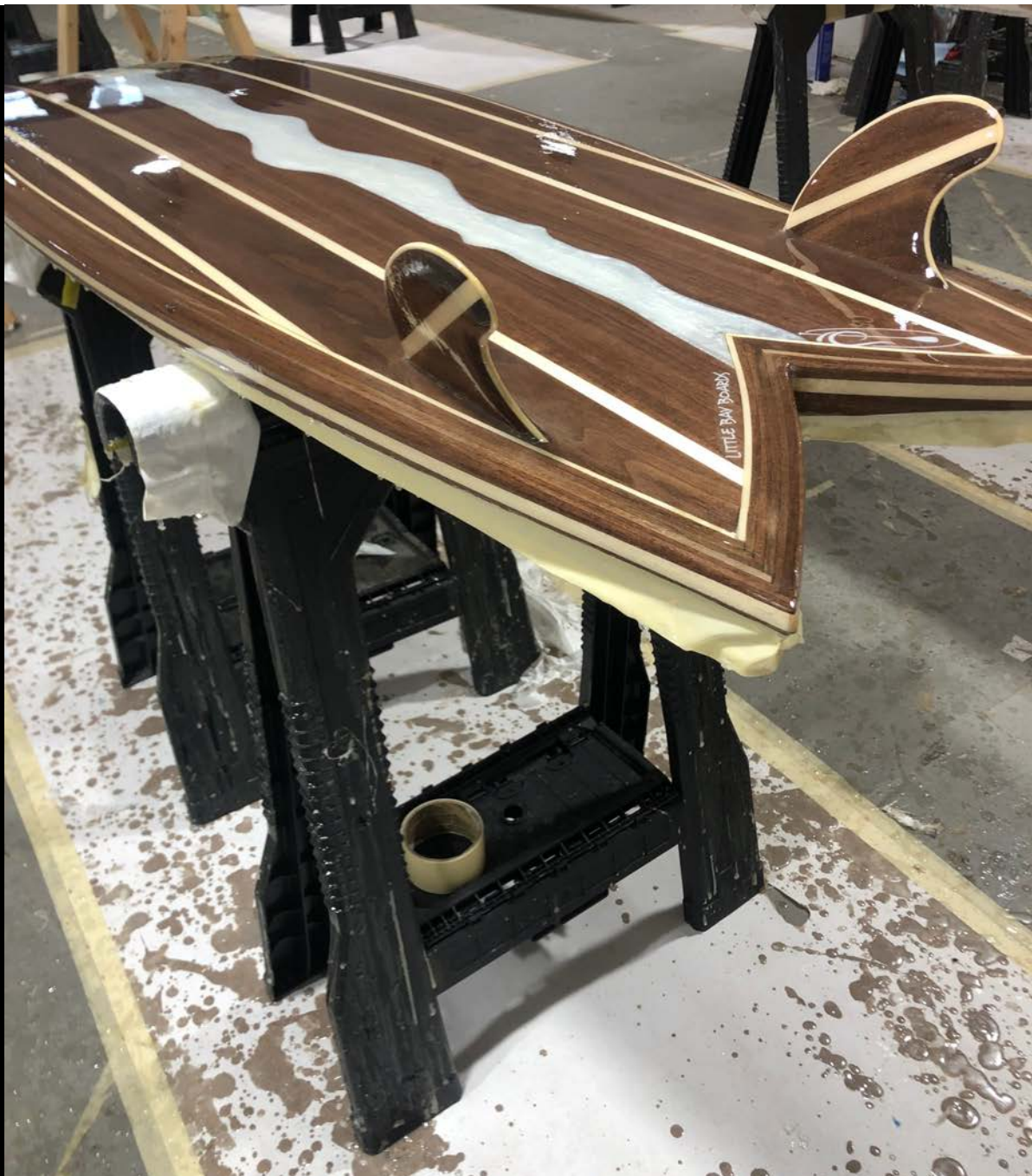
Final coat of epoxy...
